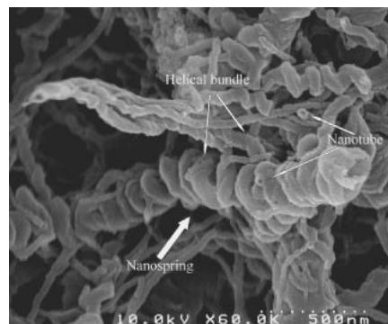
Fig. 5. FE-SEM image of silica obtained by sol-gel transcription method using gelator 10mimClO 4 .
