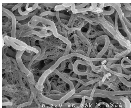
Fig. 3. FE-SEM image of xerogel prepared from t -butyl alcohol gels of 11pyClO 4 (concentration: 50 mg/0.5 mL).
